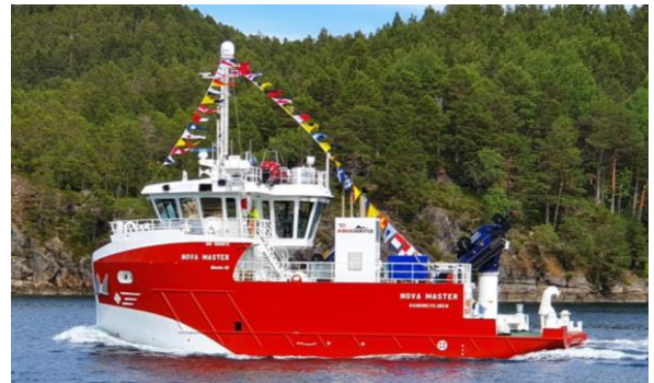
MACHO 25 DE – NOVA MASTER Yard Sletta Verft Y.no 171 Gearbox 2G23-35F Propeller P58.19.240.4D - HS E-motor 2 x 374 kW-1500 rpm
