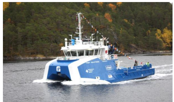
MACHOCAT 25 – FRØY VALKYRIEN Yard Sletta Verft Y.no 158 Gearbox 2 x G35F Propeller 2 x P39.13.170.4D HS E-motor 2 x 375 kW-1800 rpm
