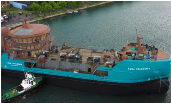
AQUA CALEDONIA Yard Balenciaga, Y.no. 414 Gearbox G60FP Propeller P78.26.300.4D HS E-motors 2 x 900 kW – 1500 rpm (tot.1800 kW)
