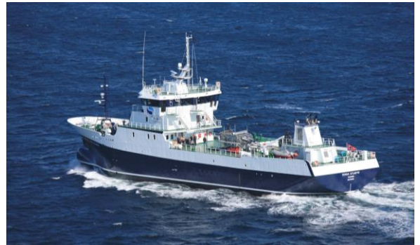
RONJA HARVESTER & RONJA ATLANTIC Yard Aas Mek. Verksted AS. Gearbox GXU600FK Propeller P85.26.280.4D Engine 1920kW-1600 rpm
