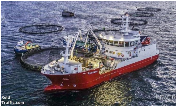
AQUA VIKING (Ex MARTIN SÆLE) Yard Gondan – Spain, Y.no 468 Gearbox G70FK Propeller P78.26.300.4D HS Engine 1920 kW-750 rpm
