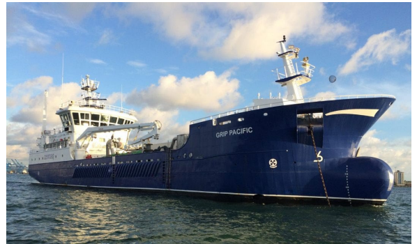
GRIP PACIFIC Yard HAT-SAN TURKEY Gearbox G60FK Propeller P78.26.300.4D HS Engine 1730 kW-900 rpm
