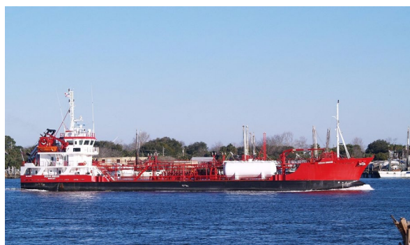
OCEAN BREEZE Yard Aas Mek. Verksted AS Gearbox 2 x G30K Propeller 2 x P39.15.160.4D Engine 2 x 537kW-1800rpm
