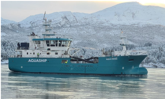
AQUASHIP (Ex MARTIN SÆLE) Yard Gondan – Spain, Y.no 468 Gearbox G70FK Propeller P78.26.300.4D HS Engine 1920 kW-750 rpm
