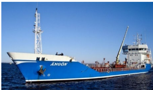
ÄNGÖN Yard Naval Shipyard Gdynia Gearbox G60FK Propeller P85.28.300.4 – DNV ICE 1B Engine 1310kW-825rpm
