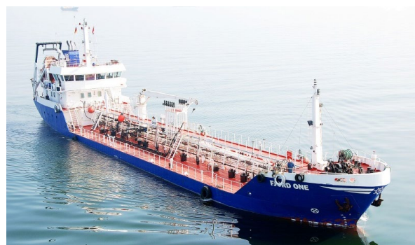
FJORD ONE Yard Ö-varvet AB Gearbox G42F Propeller P50.17.210.4 Engine 940kW 1600rpm
