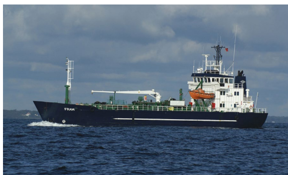
FRAM Yard Ö-varvet AB Gearbox G50FKV Engine 956kW-1600rpm
