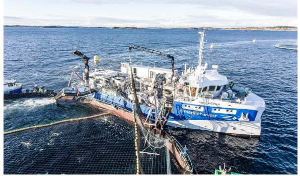
MACHO 40 – FRØY FIGHTER Yard Sletta Verft Y.no 150 Gearbox G50FKV – 2 x PTO Propeller P58.19.240.4D - HS Engine 735 kW-1800 rpm
