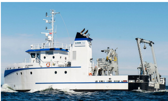
R/V VIRGINIA Yard Méridien Maritime Réparation Gearbox 2G27-42FK – 2 x PTO Propeller P60.20.195.5D – 5 BLADE CPP Engine 2 x 492 kW- 1800 rpm
