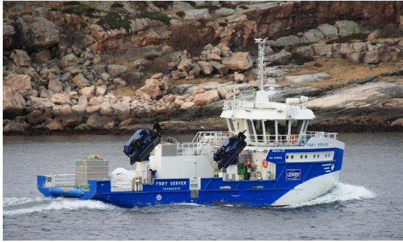
MACHO 25 – FRØY SERVER Yard Sletta Verft Y.no 145 Gearbox G50FKV – 2 x PTO Propeller P58.19.240.4D - HS Engine 735 kW-1800 rpm
