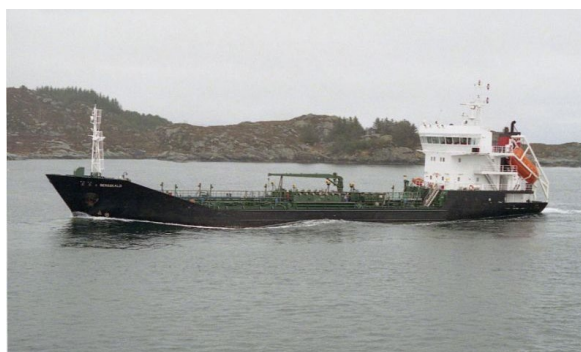
SENJA Yard Stocznia Marynarki Gearbox G60FK Propeller P85.28.300.4 - DNV ICE 1B Engine 1310kW-825rpm
