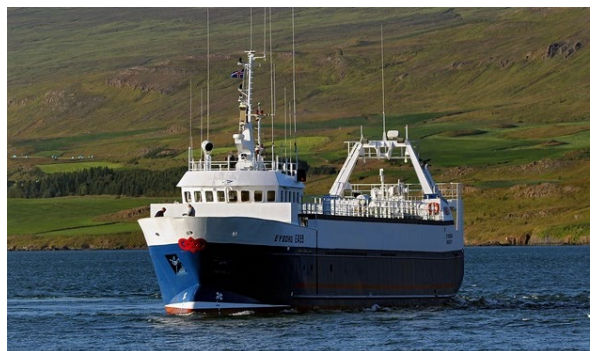
HAUKAFJELL, THINGANES, AESKAN & EYBORG Yard Carnave Shipyard Gearbox G50FK Propeller P70.22.250.4D Rudder nozzle RD250x0,5 19A Engine 730 kW-900rpm
