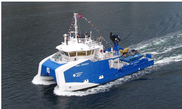
MACHOCAT 25 – FRØY HARVEST Yard Sletta Verft Y.no 157 Gearbox 2 x G35F Propeller 2 x P39.13.170.4D HS E-motor 2 x 375 kW-1800 rpm
