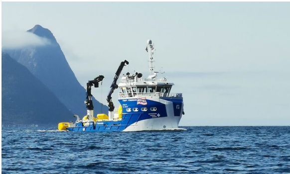
MACHO 25 DE – FRØY FINNMARK Yard Sletta Verft Y.no 169 Gearbox 2G23-35F Propeller P58.19.240.4D - HS E-motor 2 x 374 kW-1500 rpm
