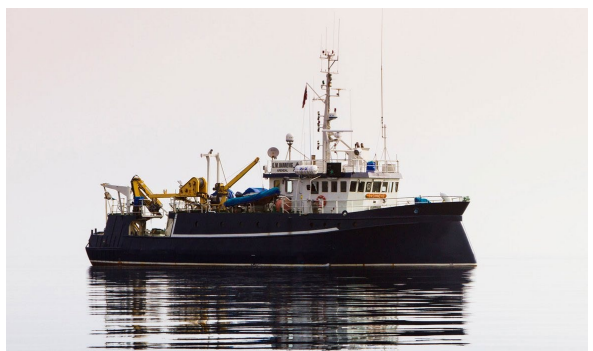
R/V G. M. DANNEVIG Yard Kystvågen Verft A/S Gearbox 2G27-42F Propeller Engine 2 x 250kW-1800rpm
